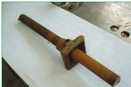
>> Spindle and nut with severe rust and corrosion
